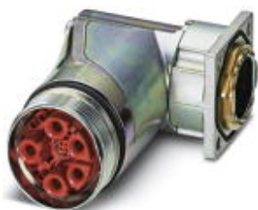
Device connector for front wall, SB, angled rotatable, shielded: yes, for standard and SPEEDCON interlock, M40, No. of pos.: 4+4+4+PE, type of contact: Socket, Crimp connection, Axial O-ring, 4x Ø4,2
