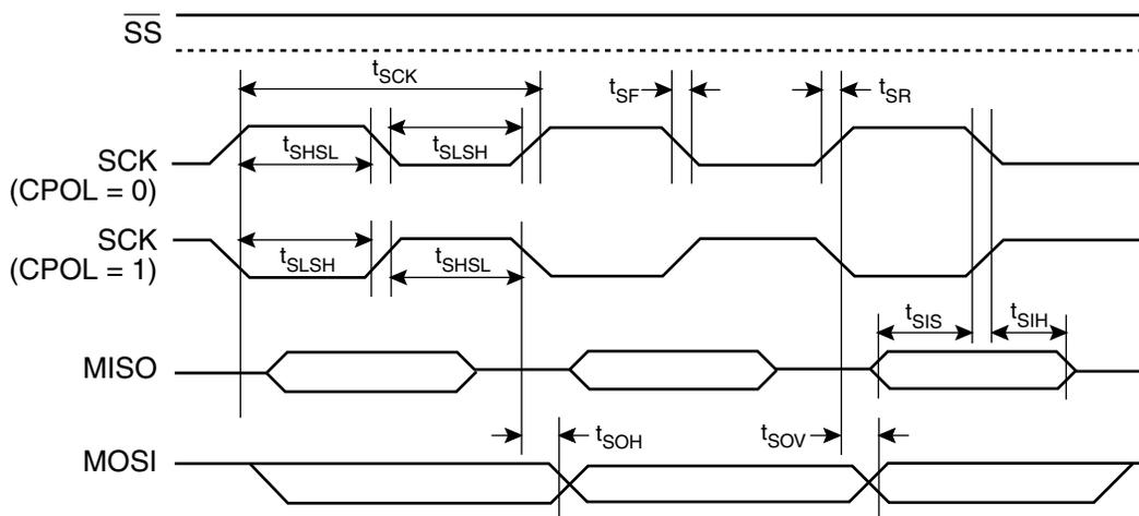
Figure 14-7. SPI Slave Timing (CPHA = 1)
