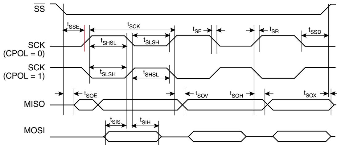
**Figure 14-8.** SPI Transfer Format with CPHA = 0
