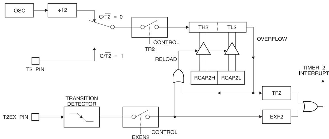
**Figure 10-3.** Timer 2 Auto Reload Mode (DCEN = 1)
