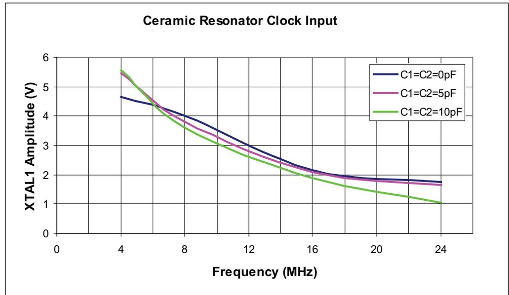
Figure 16-5. Ceramic Resonator Clock Source (B)
