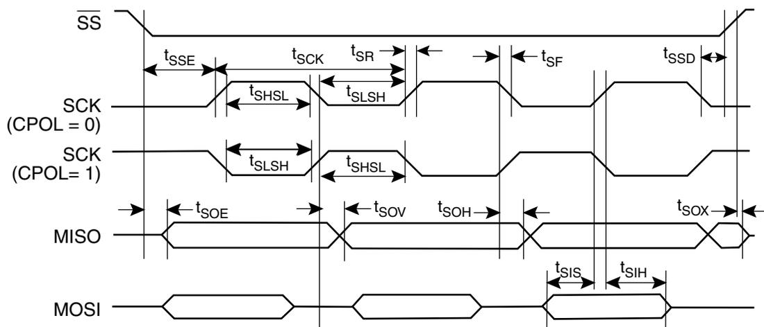
Figure 14-6. SPI Master Timing (CPHA = 1)
