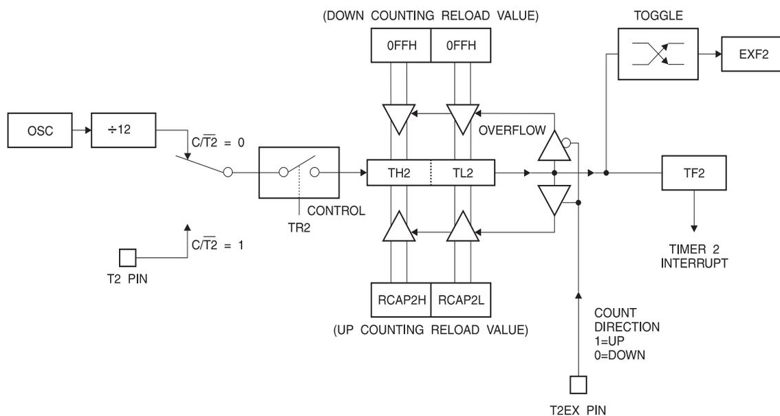
**Figure 10-4.** Timer 2 in Baud Rate Generator Mode
