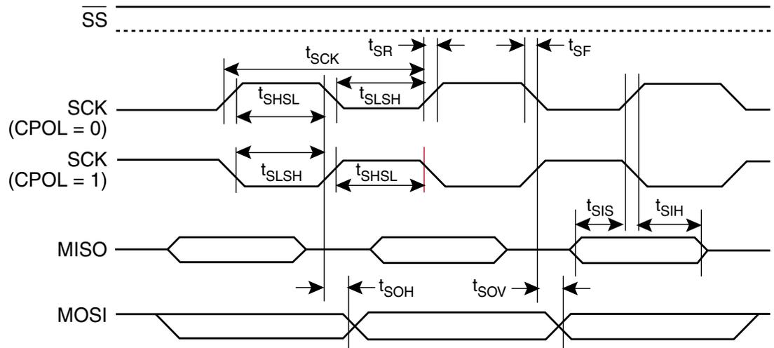
Figure 14-5. SPI Slave Timing (CPHA = 0)
