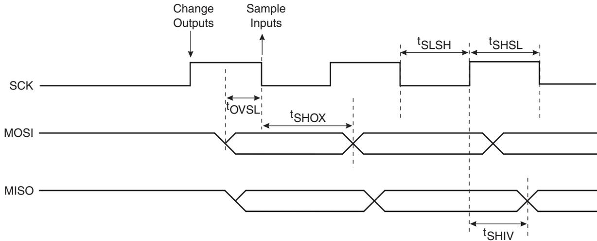
Table 28-1. Serial Programming Characteristics,  $T_A = -40^\circ\text{C}$  to  $85^\circ\text{C}$ ,  $V_{CC} = 2.7\text{V} - 5.5\text{V}$  (Unless Otherwise Noted)
